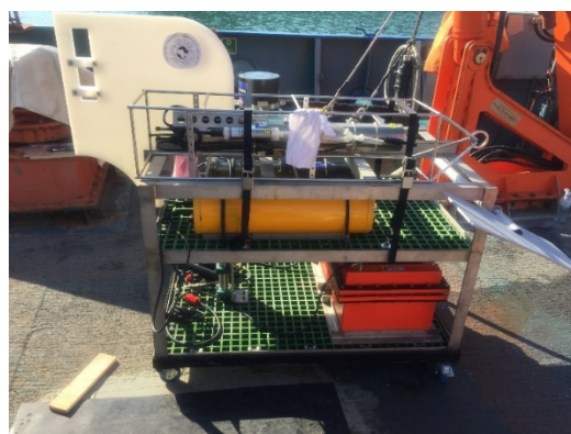
Fig. 2 Deep-tow magnetic system
